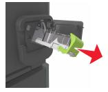
Use the metal tab to lift the staple guard, and then remove any loose staples.
